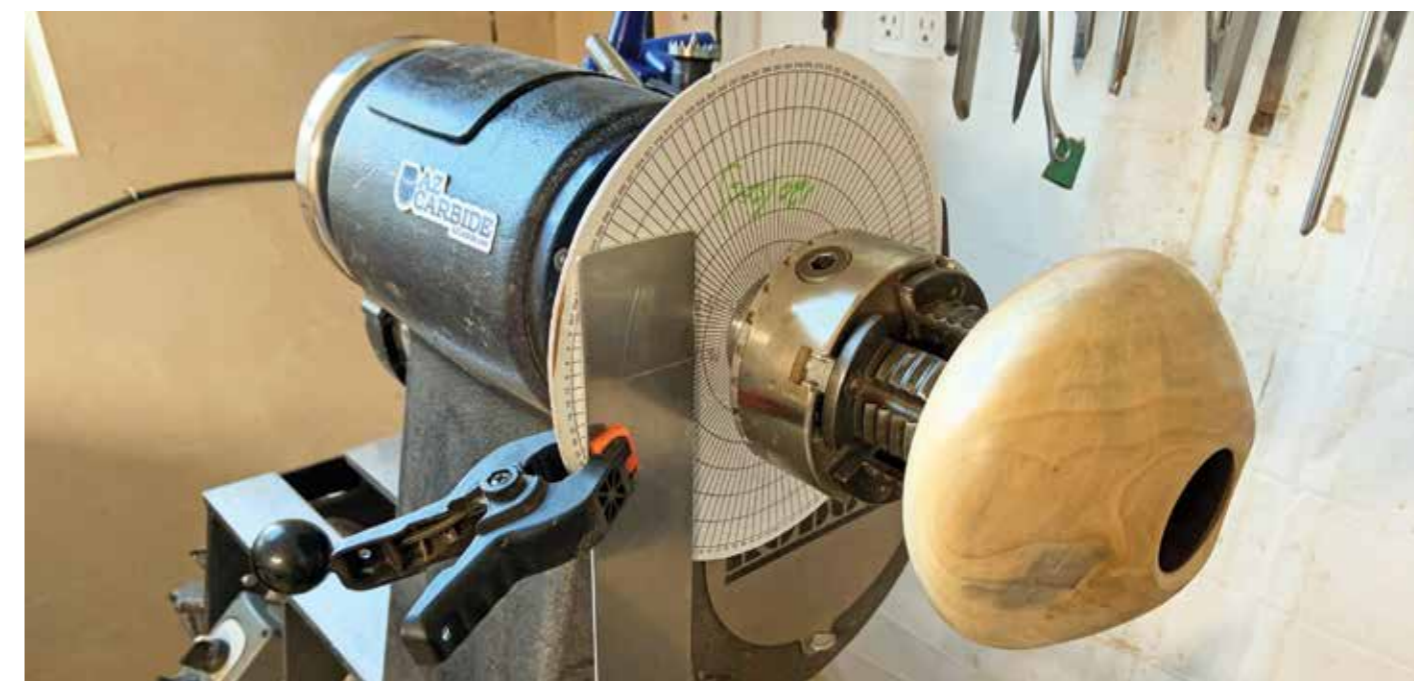
Homemade index wheel using polar graph paper and shop clamps
